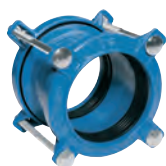
Series 601 Supa® straight coupling universal for uPVC, AC, steel, cast iron and ductile iron pipes DN40-400 PN16 Ductile iron
