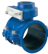
Series 727/10 Tapping saddle for underpressure drilling For PE and PVC pipes DN80-200 Ductile iron
