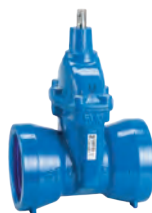
Series 33/00 Gate valve with socket ends for cast iron pipes DN80-300 PN16 With internal enamel Ductile iron
