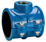
Series 10/00 Tapping saddle for uPVC and PE pipes DN50-300 Lower part in stainless steel from DN250 Ductile iron
