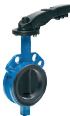
Series 820/00 Butterfly valve Centric with loose liner Wafer type DN25-1000 PN10/16 Ductile iron
