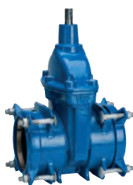
Series 01/70 Supa Plus™ gate valve Tensile for PE and uPVC pipes DN40-300 PN16 Ductile iron
