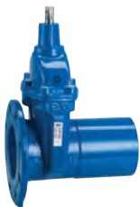
Series 12/51 Gate valve with flange/spigot end for cast iron pipes DN50-300 PN10/16 Ductile iron
